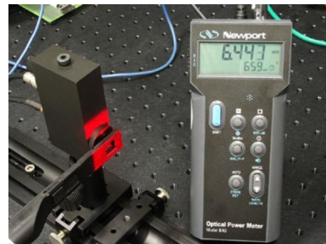
Figure 14: Newport sensor in the center of the homogenised laser light
